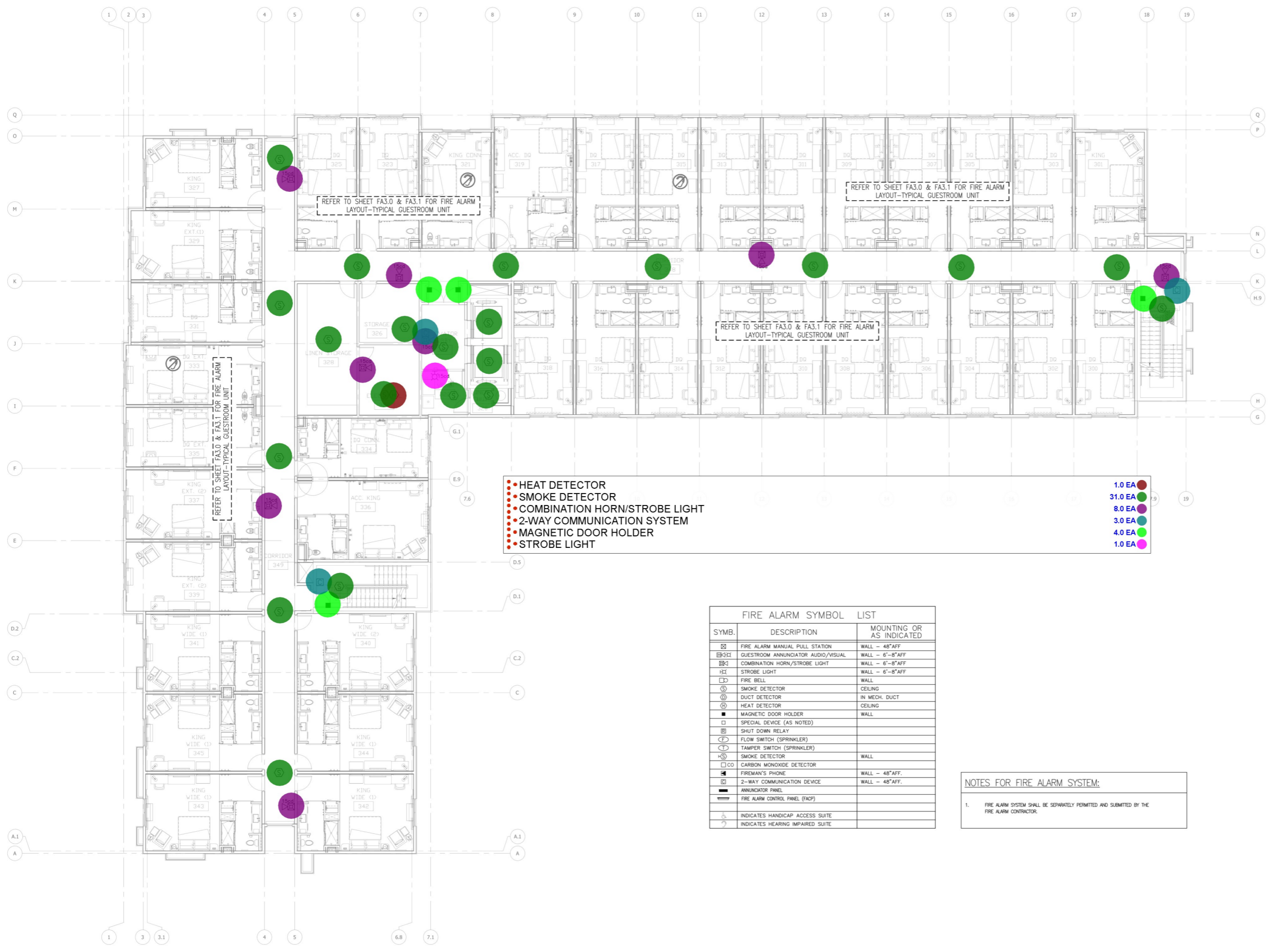
1 FIRE ALARM THIRD FLOOR PLAN SCALE: 1/8"=1'-0"
